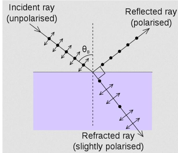
Figure 2: Illustration of the Brewster's angle and the polarization of the reflected light beam.
