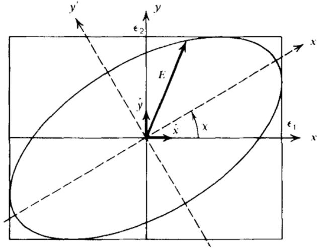
Figure 1: The polarization ellipse. Credit: Figure 2.4 from Rybicki & Lightman (2004).
