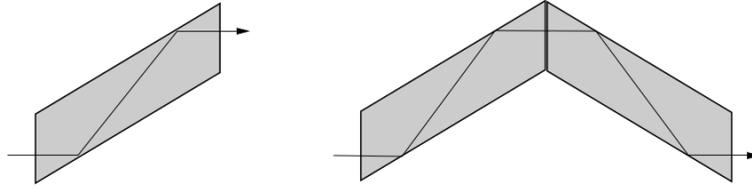
FIGURE 8. Traditional arrangements for quarter-wave (left) and half-wave (right) Fresnel rhombs.
