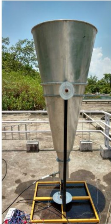
FIG. 3: Dimensions (in mm) of the dual-mode horn are shown on the left. Note the step discontinuity in the horn flare, which generates a second mode. The horn is fed using an N-type coaxial connector. On the right is the constructed horn fixed on an altitude-azimuth mount. Scales are added for pointing the antenna in a particular direction. A mobile phone running an appropriate application for showing the azimuth and elevation values can also be alternatively fixed on the system for pointing
