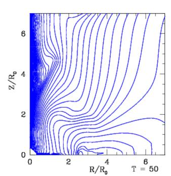
Poloidal magnetic field lines for the different timesteps. Initial stages in the simulation are related to the reshaping of the magnetic field, because of reconnection. In our simulations resistivity facilitates reconnection, so that in effect result depends on resistivity in the magnetosphere.
