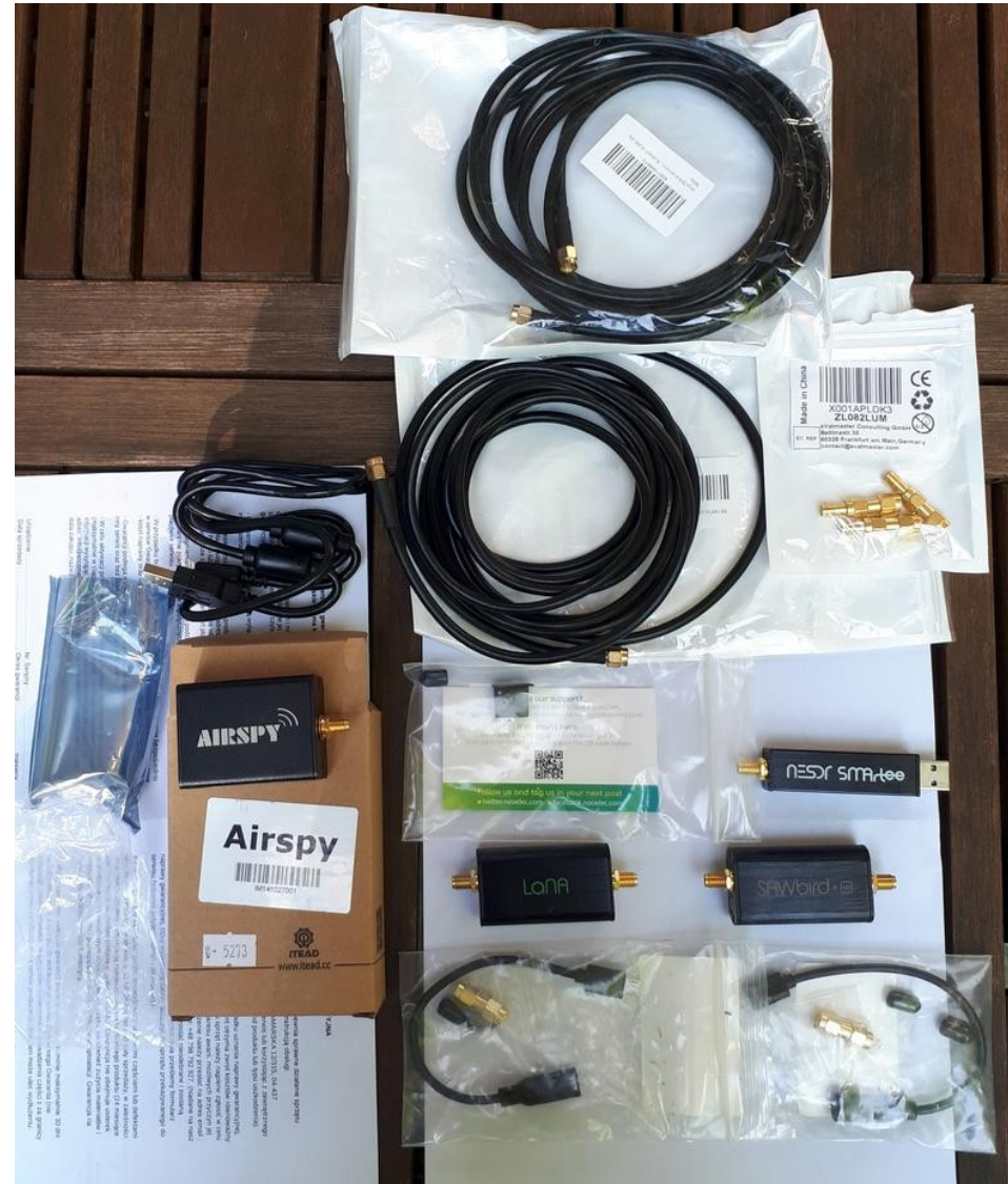
Airspy R2 + LNA SAWbird+H1 filters:
